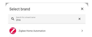
Select "Add Zigbee device," and HA will begin searching for Zigbee devices and add Linxura smart controller to Zigbee network.
